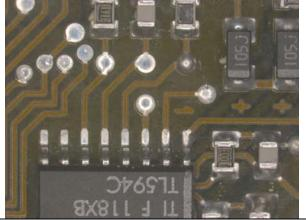
**LED3000 RL with Diffusor**The reflections at the solder joints are strongly reduced.
