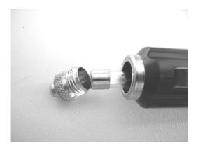
Replace the miniature fuse with the replacement provided by unscrewing the base contact to the europlug. After replacement, screw the base contact on again.
