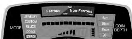
In ZERO Mode, the discrimination pattern shows all 12 pixels are on.
