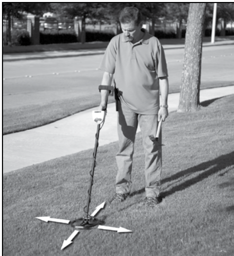
Traditional pinpointing technique using Pinpoint pushbutton.
