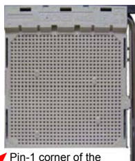
Pin-1 corner of the CPU socket
