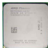
Pin-1 triangle marking of CPU
