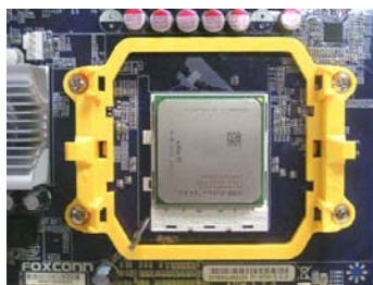
2. Align pin one of the CPU with the CPU socket, and gently put the CPU onto the socket.
