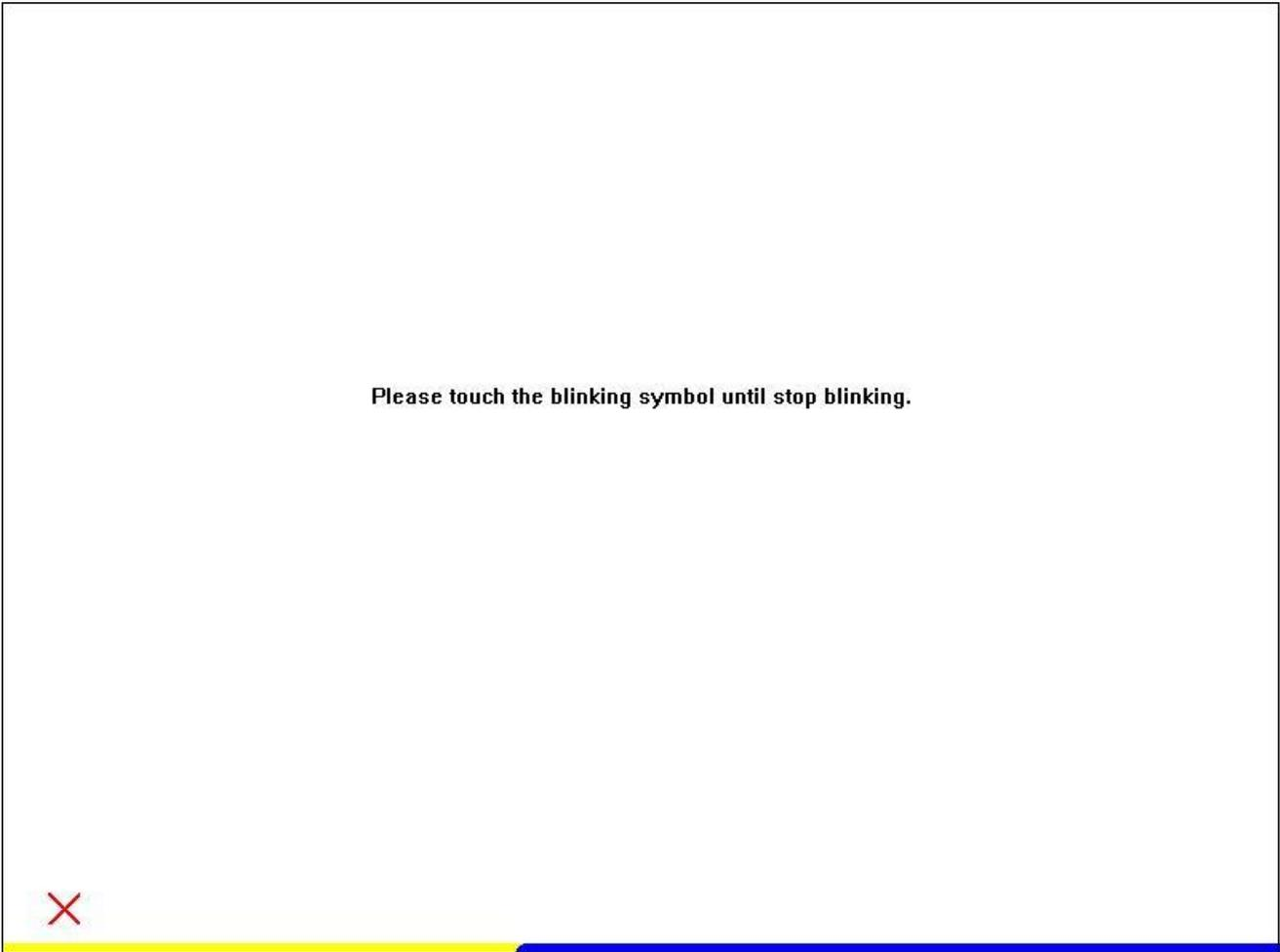
**The screen will show as above picture, use the Touch pen to point on dot and align the cursor, if the actual alignment has too much difference then the system will skip back to previous screen and require calibration again.**
