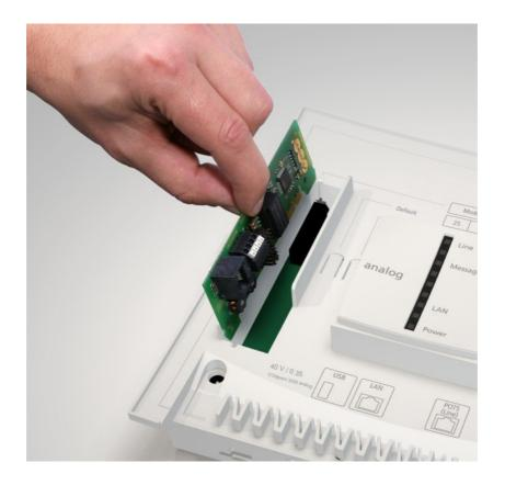
The figure in the following shows the position of the module slot under the cover panel, as well as the plug-in connection of the module.
