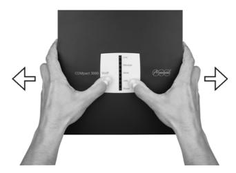
3. Lift the upper cover panel vertically off the casing. To support this action, press with the thumbs against the casing.
