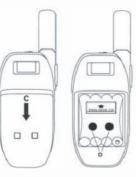
• Mount the battery compartment cover and the belt clip.
