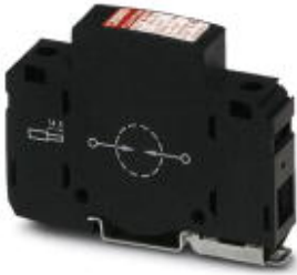
Type 1 / Class I / B arrester (lightning current arrester) with encapsulated arc chopping spark gap, 1-channel. Housing width: 17.5 mm (1 Div.)
