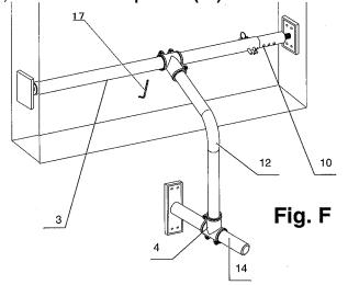
NOTE: /! The wall must be strong enough to hold a load of 100 kg. The pipe Nr. 3 and Nr. 10 must be parallel to the window-sill, and must be pressed in tightly. T Clamp 4 must be tightly screwed on to 12 and 14. If the side walls are not strait, you must even out the sides so that the support plates (2 and 9) are parallel to the wall.
