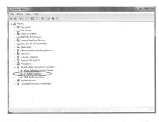
In the Device Manager Crick on the +imaging devices conectly you should see the "STK1160 Grabber". If it has a Yellow mark next to it then this means that the driver is not installed correctly. You will need to remove the driver and disconnect the Easy CAP USB 2.0 Video Adapter with Audio from the computer and reconnect is to install the driver again.
