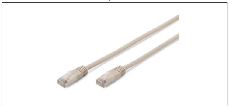
CAT 5e F-UTP patch cable, Cu, PVC AWG 26/7, length 10 m, color grey
