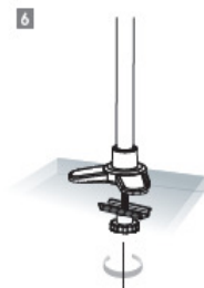
The Hand Drive Screw and Grommet Clip from the bottom of the desktop through to Grommet module, tighten the fixed. 將手旋螺絲及Grommet夾片由桌面底部穿進Grommet底座裝緊固定。
