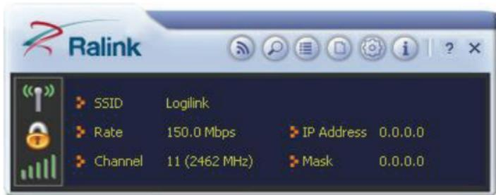
*The Ralink wireless utility starts in compact mode as shown above, provides profile management, the available networks listing, a statistical counter display, Wi-Fi multimedia (WMM), protected Wi-Fi setup, Cisco compatible extensions (CCX), call admission control (CAC), radio controls, Ralink driver/utility information, and*
