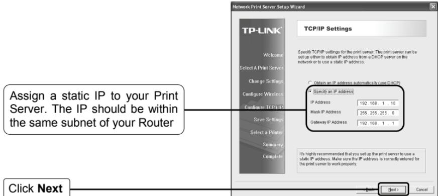
**Note** The IP address of the print server must be within **the same subnet** with your Router, for example:
