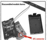
below. Be careful when switching on the transmitter Aurora 9, the module is not switched on as long as the transmitter is not in transmitting mode. You will recognize the switch-on state of the module when the red LED starts blinking. The blinking red LED on the module indicates communication between module and transmitter. At the transmitter working in Duplex mode moreover a green LED will turn on.
