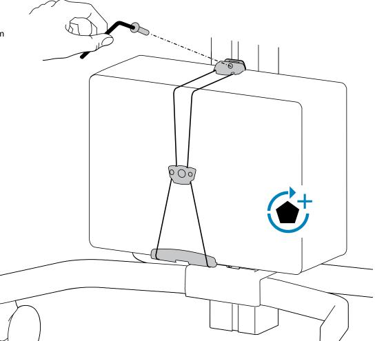
**15** NOTE: Leave enough slack in cable to allow full range of motion.
