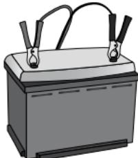
2. Connect the charger's red cable clamp to the battery's positive terminal post (+), and the black cable clamp to the battery's negative terminal post (-).
