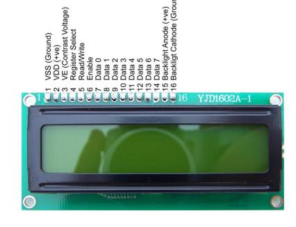
The LCD controller gives us two ways to send data: in one-byte (8 bit) chunks, or as two consecutive nibbles (4 bit). The second approach seems more complicated, but very frequently used. Why? It simplifies the hardware, and lets us talk to the LCD with half as many data lines. In general, I/O lines are a scarce resource! We use the 4-bit method on this board, and need only 6 I/O lines (2 control + 4 data) to communicate with the LCD.
