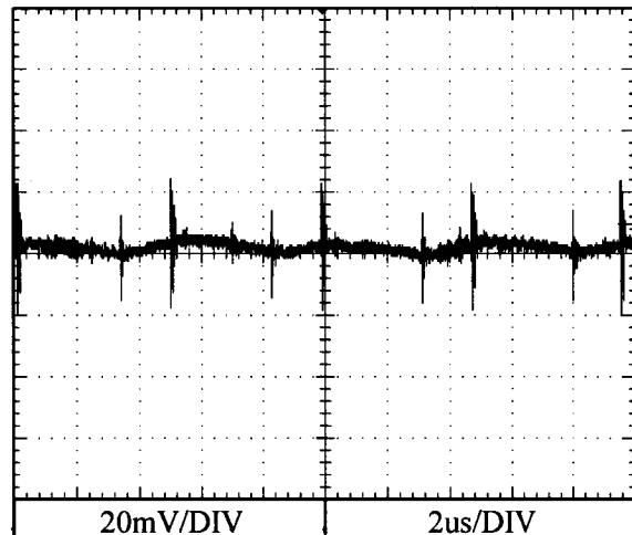
**2.18 Output ripple and noise waveform**
