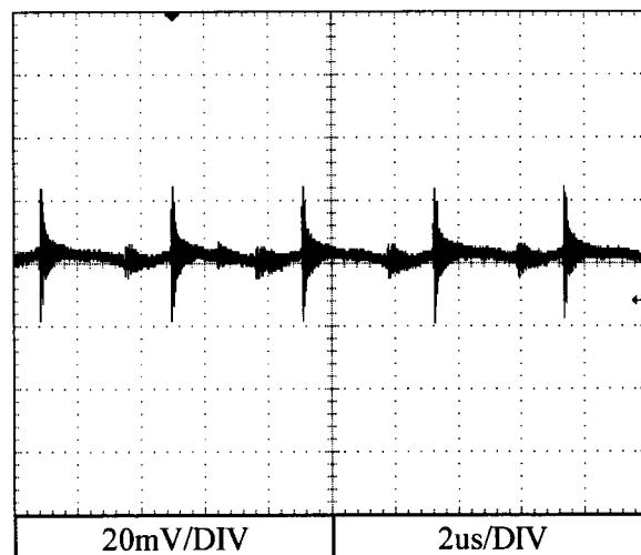
**2.18 Output ripple and noise waveform**Conditions; Vin : 115VAC
