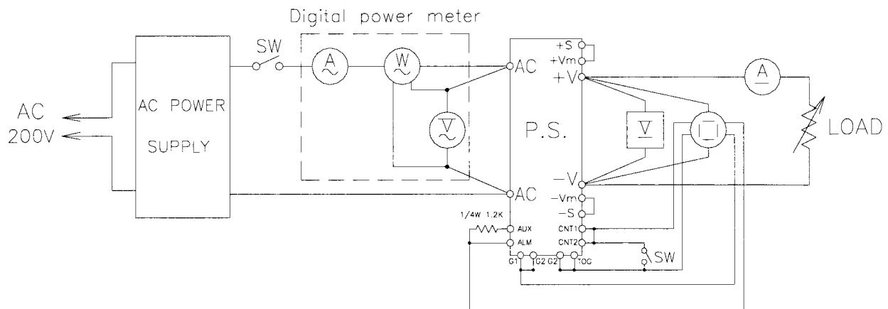
(8) Output fall characteristics with ON/OFF CONTROL
