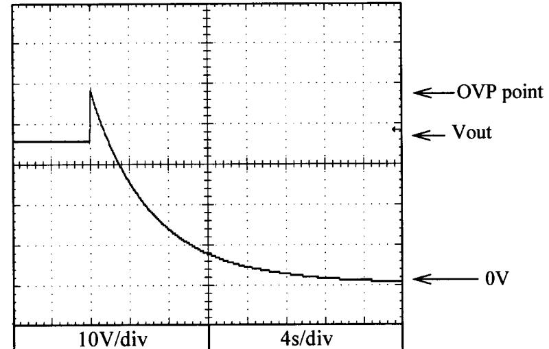
**2.4 Over voltage protection (OVP) characteristics**
