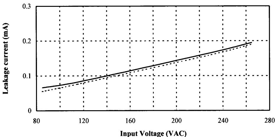
**2.17 Leakage current characteristics**
