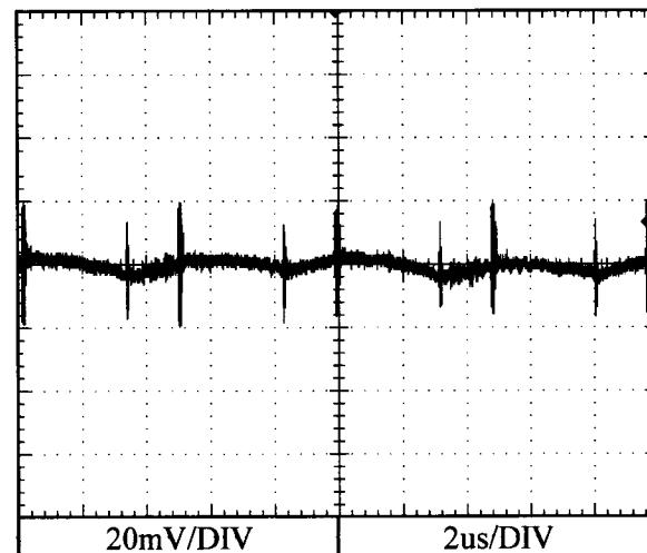
**2.18 Output ripple and noise waveform**
