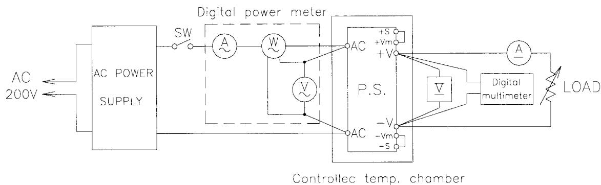
**(4) Over voltage protection (OVP) characteristics**
