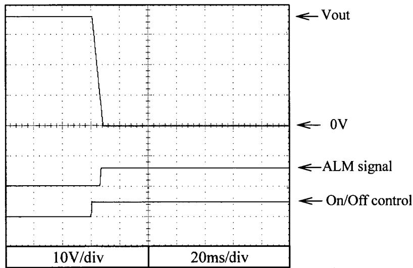
**2.8 Output fall characteristics with On/Off control**
