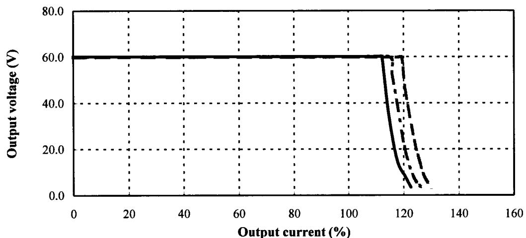
**2.4 Over voltage protection (OVP) characteristics**
