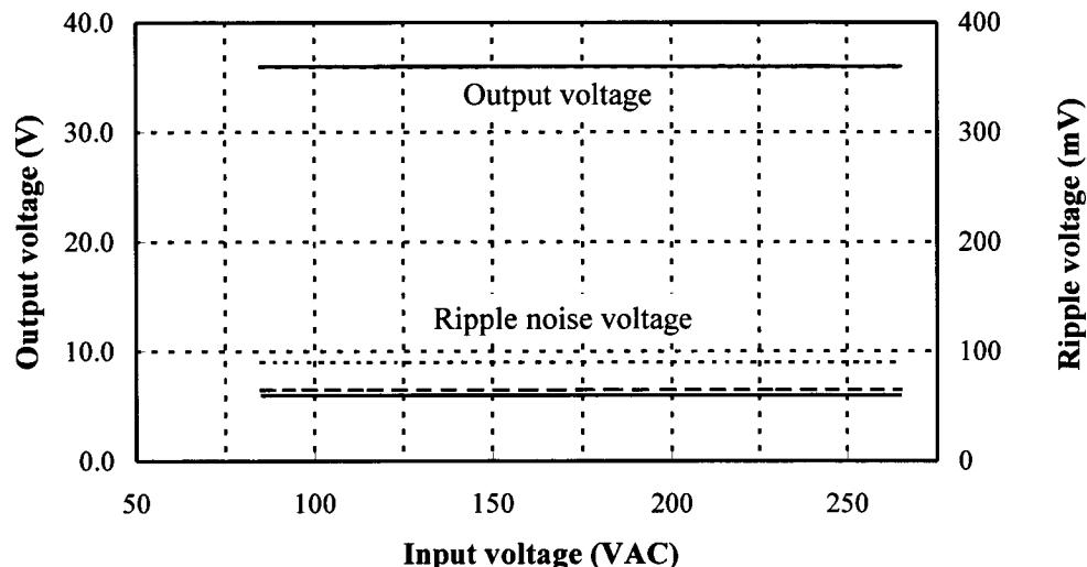
**2.1 Steady state data****(2) Output voltage and Ripple voltage v.s. Input voltage**
