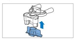
3 Close the spring to lock the two parts together.
