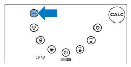
The descaling cycle is in progress. During the descaling cycle, the descaling solution comes out of the machine in intervals. During the last 5 minutes the descaling solution flows continuously.
