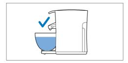
10 Fill the water reservoir with fresh tap water and place it back onto the machine.
