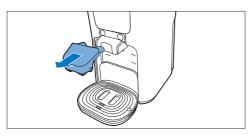
3 Remove the top part of the milk spout from the bottom part by pulling it firmly.
