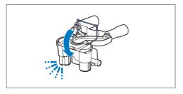
4 Place the frothing system in the bottom part of the milk spout.
