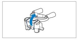
Remove the inside part of the frothing system by pulling it downwards.
