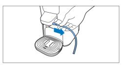
2 To remove the milk spout from the machine, pull it towards you.
