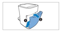
Slide the milk spout onto the machine. Make sure you attach the milk spout by sliding it over the guiding rails on the coffee spout. You hear a click sound when the spout is attached properly.
