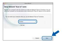
The name you type will appear in the **Destination** drop-down list in **Scan to Network Device** from the **Scan** tab in Web Based Management (ADS-1100W only) (see the *User's Guide*) or on the LCD of the machine (ADS-1600W only) when you choose a scan option. For more information, see the *User's Guide*.
