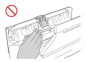
DO NOT carry the machine by holding the top cover. Doing this may cause the machine to slip out of your hands. Only carry the machine by placing your hands under the entire machine.
