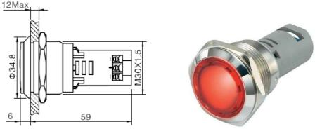
12 MAX: means the panel thickness, the max thickness for the panel no more than 6mm.
