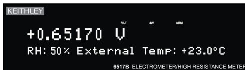
Figure 7: Relative humidity and external temperature display
