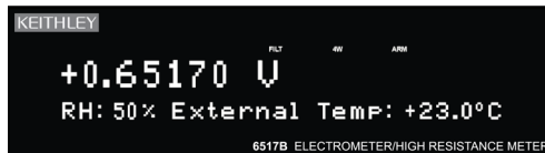
Figure 43: Relative humidity and external temperature display
