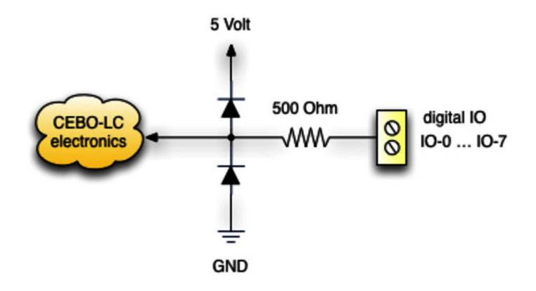
\* Single I/O only. Total current should be limited to less than 25 mA.
