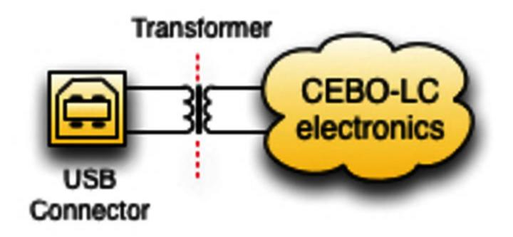
The isolation is rated 500 Volt / 60Hz (1.000 VDC for one second).
