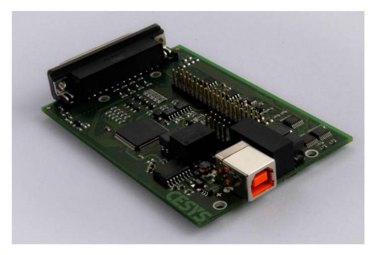
CEBO-LC is also available as "OEM-version" without the enclosure and without screw terminals. The screw-terminal signals are on a 2x20 pin standard 0,1" (2,54 mm) header instead. Use the OEM version to embed CEBO-LC functionality into your machines or devices.
