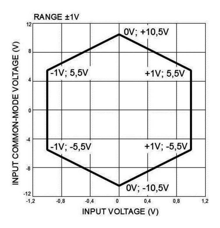
Example: You have two voltages (5V & 11V) relating to mass.  $V_{in} = 6V \& V_{cm} = 8V$ This point is in no figure inside the hexagon, so you get no valid reading.
