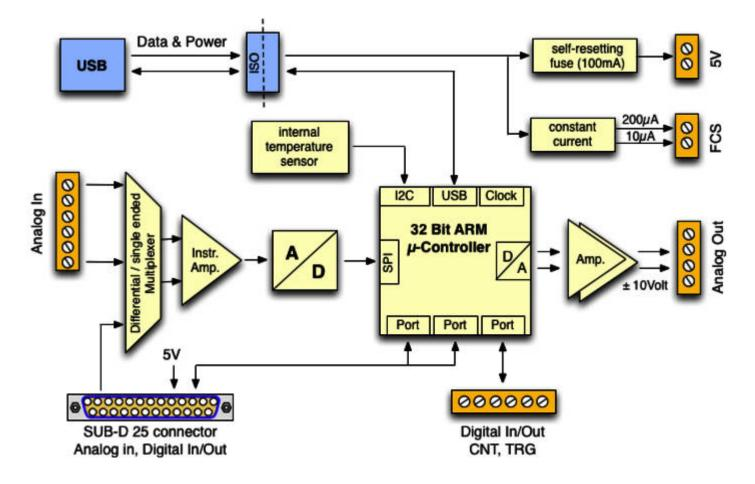
Figure: simplified block diagram
