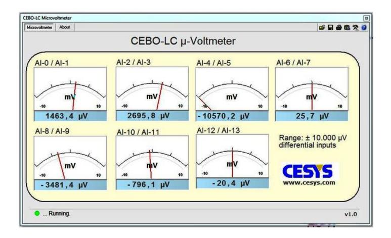
The CEBO-LC Microvoltmeter has 7 differential inputs. The measurement range is 10 mV.
