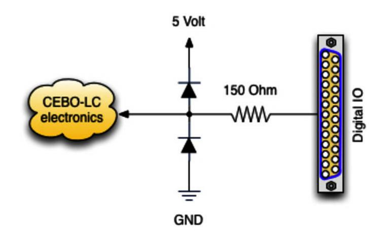
\* Single I/O only. Total current should be limited to less than 25 mA.
