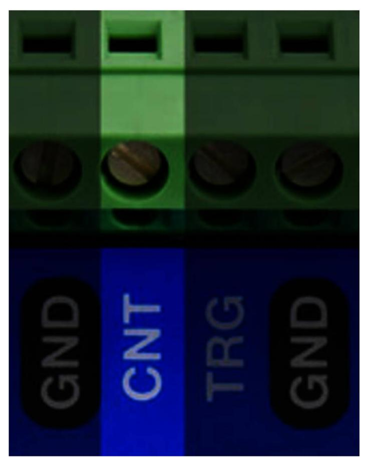
CEBO-LC has an external counter input. It is located at the screw terminal labeled CNT.
