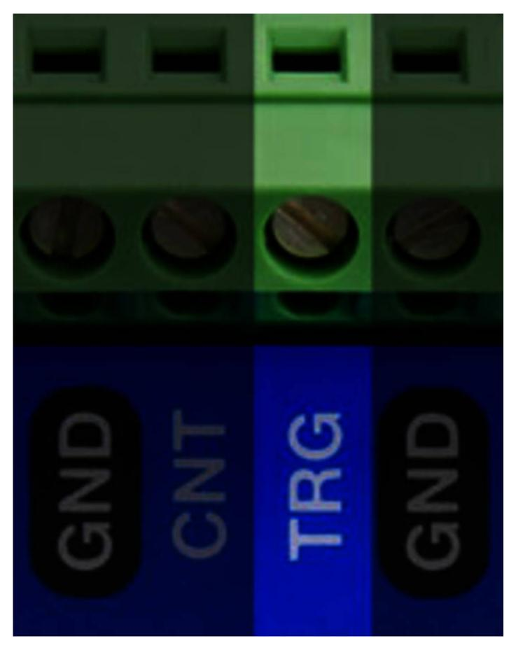
CEBO-LC has one Trigger Input/Output which is located at the TRG terminal. With firmware releases 1.x, the
