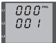
Fig. Programming mode Parameter display The individual parameters can be changed using buttons 1 and 2 (cf. page 48).
