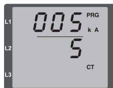
Fig. Current transformer programming mode The primary and secondary currents can be changed using buttons 1 and 2 (cf. page 39).
