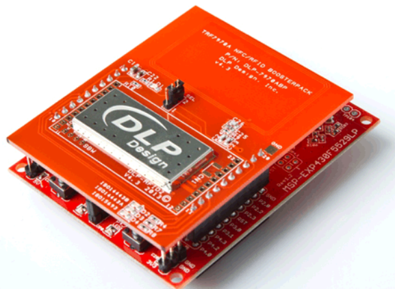
Figure 37. F5529 LaunchPad With DLP-7970ABP NFC BoosterPack
