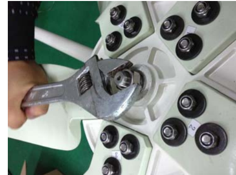
③ Fully tighten the nut to 154N.m
