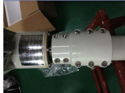
⑤ The pole is inserted into lower part of the clamp.
