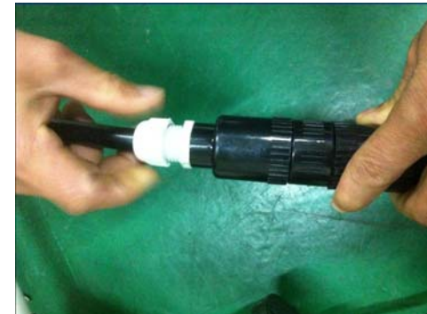
⑥ Screw up the waterproof cover.
