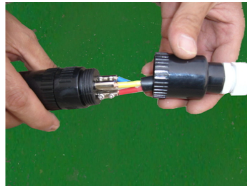
⑤ Screw up the cable cover.
