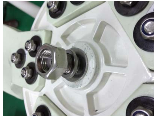
② Place the hub with blades onto the rotor shaft and "spin" it completely onto the turbine alternator shaft, then place in sequence of flat washer, spring washer and hex nut.
