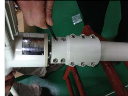
⑥ tighten the nut to 9N.m
