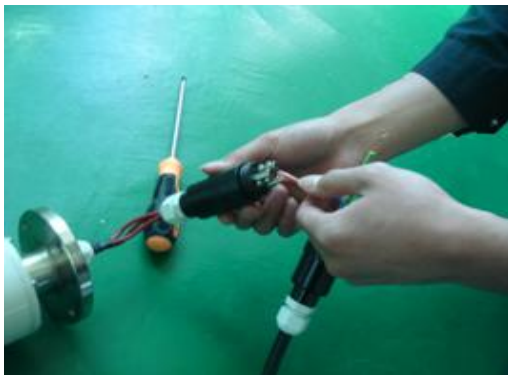
④ Connect the three-phase lead wires into the terminals (make sure three phases are not short circuited)
