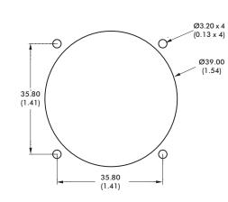
The joystick is dropped into the panel cut-out. For panel thickness of <3mm, M3 x 16 countersunk machine screws are recommended. Please note: Image (left) shows a square bezel, a circular bezel is also available for this option.
