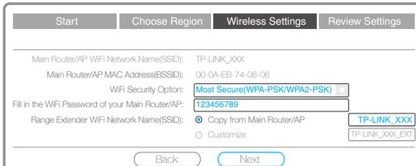
c. Fill in the **Wi-Fi Password** of your main Router/AP. The TL-WA860RE's **Wi-Fi network name (SSID)** can be copied from your main Router/AP name (**TP-LINK\_XXX**) OR BE CUSTOMIZED A NEW ONE (**TP-LINK\_XXX\_EXT**).
