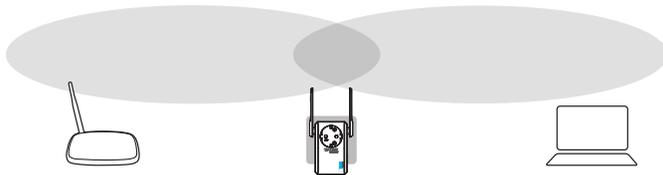
Generally, the ideal location for your extender is **Halfway** between your wireless router and Wi-Fi enabled devices.
