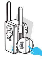
⌚ The 'Signal' LED will go from flashing green to solid green, solid orange, or flashing orange in 1 minute, showing that WPS connection has succeeded.
