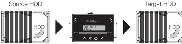
Connect a source hard disk into source port; connect a hard disk to backup into the target port. Press "O" to start to backup.
