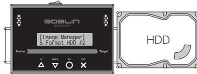
Select function table 4.Image Manager >> 5.Format HDD #2 to create the BIG MASTER HDD format. Press "O" to check information such as image names, used amount, etc.
