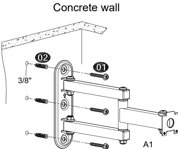
Figure 2 (keep the wall plate level)
