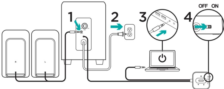
1. Plug the satellites cable into the subwoofer jack.
