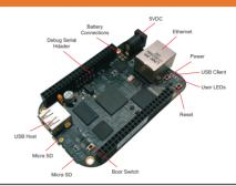
Power up the board by plugging in the USB cable provided, to connector P4 on the element14 BeagleBone Black board, and the USB port on a host system
