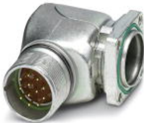
Device connector, front mounting, angled rotatable, Screw locking, M23, Number of positions: 12, Type of contact: Male connector, Crimp connection, Axial O-ring, 4xØ3,2, shielded: Yes, Flange dimensions: 26 mm x 26 mm
