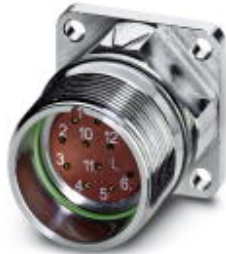
Device connector, front mounting, straight, Screw locking, M23, Number of positions: 12, Type of contact: Socket, Crimp connection, Axial O-ring, 4xØ3,2, shielded: Yes
