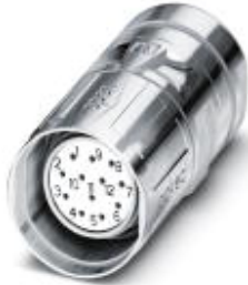
Cable connector, straight, shielded: Yes, SPEEDCON locking, M23, Number of positions: 17, Type of contact: Socket, Crimp connection, Cable diameter: 6 mm ... 10 mm
