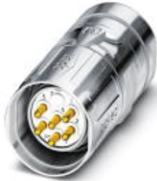
Cable connector, straight, shielded: Yes, SPEEDCON locking, M23, Number of positions: 6, Type of contact: Male connector, Crimp connection, Cable diameter: 6 mm ... 10 mm
