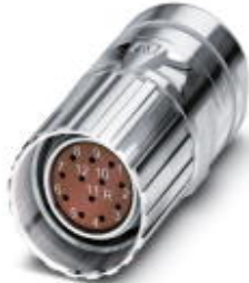
Cable connector, straight, shielded: Yes, Screw locking, M23, Number of positions: 17, Type of contact: Socket, Crimp connection, Cable diameter: 3 mm ... 14.5 mm
