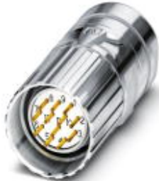
Cable connector, straight, shielded: Yes, Screw locking, M23, Number of positions: 17, Type of contact: Male connector, Crimp connection, Cable diameter: 10 mm ... 14.5 mm
