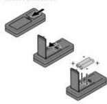
To ensure a reliable use, do not use zinc-carbon batteries Change batter-ies when battery symbol is flashing.
