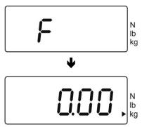
After adjustment the balance automatically returns to weighing mode. In case of an adjustment error or wrong adjustment weight "E" is displayed, repeat the adjustment process
