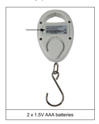
Push out the battery cover on the balance backside. Insert 2 batteries (AAA 1.5V). Reinsert the battery cover. If the batteries are empty, in the balance display appears "**LO**". Press **ON/OFF**-button and replace the batteries immediately. In order to save the battery, the balance switches automatically off after 4 minutes without weighing Deactivate this Auto-OFF function as follows:
