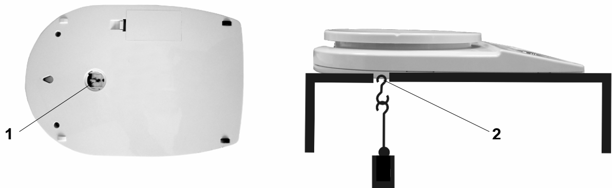
Fig. 1: Setting up the balance for underfloor weighings
