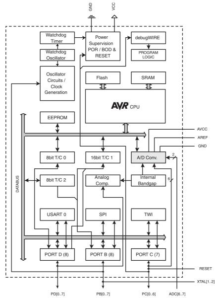
The AVR core combines a rich instruction set with 32 general purpose working registers. All the 32 registers are directly connected to the Arithmetic Logic Unit (ALU), allowing two independent registers to be accessed in one single instruction executed in one clock cycle. The resulting architecture is more code efficient while achieving throughputs up to ten times faster than conventional CISC microcontrollers.
