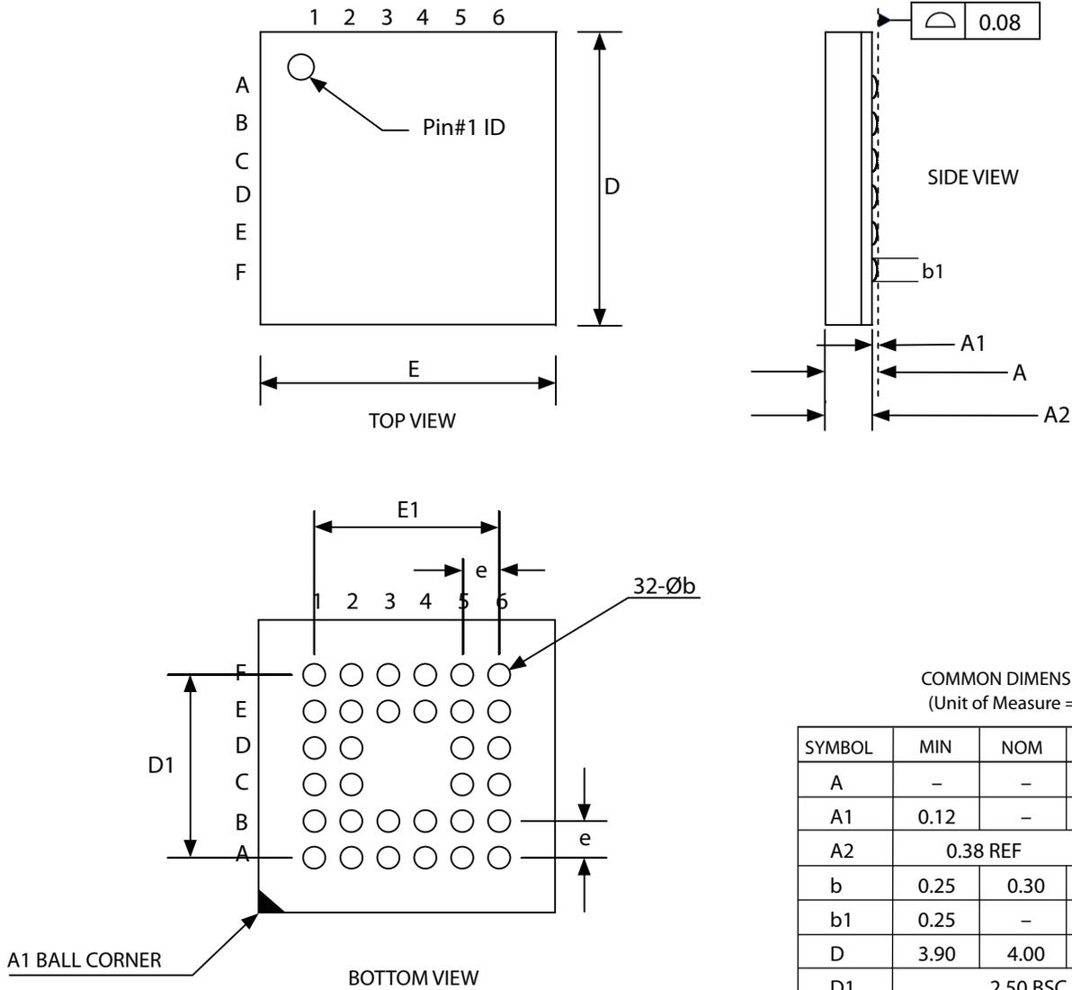
Note1: Dimension "b" is measured at the maximum ball dia. in a plane parallel to the seating plane.
