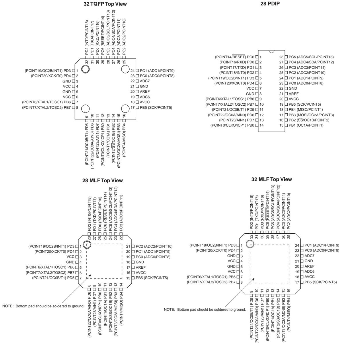
Table 1-1. 32UFPGA - Pinout ATmega48A/48PA/88A/88PA/168A/168PA
