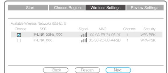
d. Select your Router/AP's 5GHz Wireless Network, for example, TP-LINK\_5GHz\_XXX.
