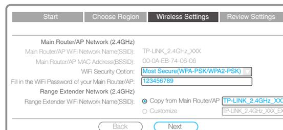
c. Fill in the Wi-Fi Password of your main Router/AP. You can copy the Wi-Fi Network Name (SSID) from your main Router/AP (TP-LINK\_2.4GHz\_XXX) or set a new one (TP-LINK\_2.4GHz\_XXX\_EXT).
