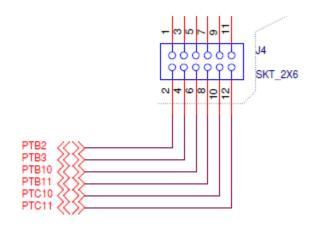
Figure 2. Swapped I<sup>2</sup>C signals Pin10 and Pin12 on J4
