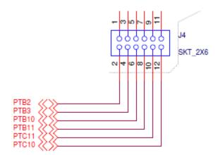
Figure 4. Correct order of I<sup>2</sup>C signals on J4
