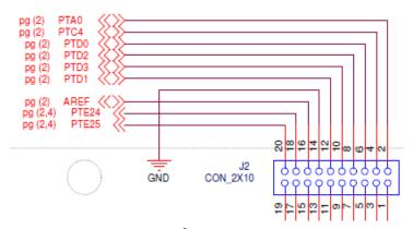
Figure 1. Swapped I<sup>2</sup>C signals Pin18 and on J2
