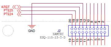
Figure 3. Correct order of I<sup>2</sup>C signals on J2
