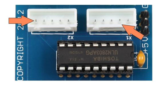
You can influence the power supply with the pin header: If you want the motors to receive their power from the Raspberry Pi, connect the two left-hand pins, marked on the following picture, with the enclosed "jumpers":
