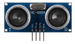
The ultrasonic module operates within a distance range of 2 to 450 cm. The maximum deviation is just 2% of the measured value. Due to the small dimensions and the high processing quality, this module is also ideally suited for mobile applications.
