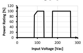
Bild 5: Derating Figure 5: Derating Figure 5: Déclassement Figura 5: Derating
